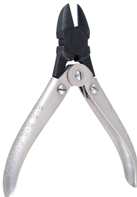
48-138-14 14 cm / 5 1 / 2 " For hard wire min. 0.87 mm / .028" upto 1.1 mm / .047" Ø max.
