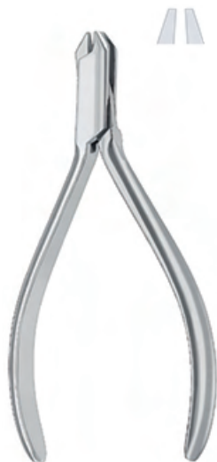
Aderer Fig. 1 48-179-11 11.5 cm - 4½" 48-180-12 12 cm - 4¾" For hard wire upto 0.7 mm / .028" Ø max.
